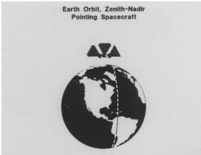
Fig. 2. Orbit of a typical Sun-synchronous satellite (9am – 9pm). The spacecraft orbit is circular at \approx 800 km above the surface of the Earth and maintains its relation with respect to the Sun-Earth line.
